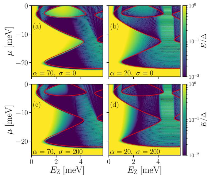
Figure 9: Phase diagram as a function of  $E_Z$  and  $\mu$  of the 3D device, with orbital magnetic field and an external superconductor included. The red line indicates the topological phase boundary. The color indicates the lowest energy of the Hamiltonian in units of  $\Delta$  on a logarithmic scale. Different panels have different parameter values for the SOI strength  $\alpha$  (in meV nm) and potential smoothness  $\sigma$  (in nm). The potential barrier height is  $V = 25$  meV.
