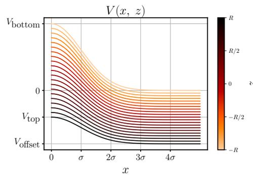
Figure 11: Potential shape inside the nanowire as given by Eq. (31). The parameter values for the simulations in Fig. 9 are  $V_{\text{top}} = -30$  meV,  $V_{\text{bottom}} = 25$  meV,  $V_{\text{offset}} = -50$  meV, and  $R = 35$  nm.
