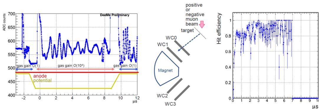
Figure 6: Output waveform of a cathode strip signal amplified through an amplifier.
