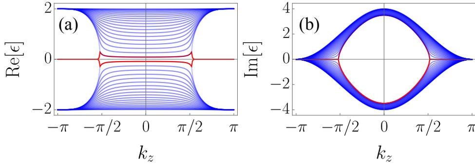
Figure 6: Real (a) and imaginary (b) part of spectra for Eq. (12) with open boundary condition in the  $y$  direction and  $k_x = 0$ . Red lines present boundary states. Here we set  $t = V = \lambda_0 = 1.0$ .
