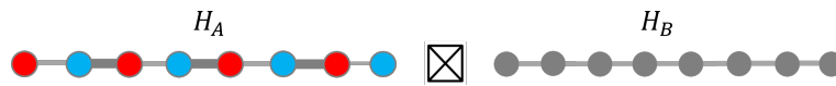
Figure 16: Tensor product structure which generates the model illustrated in figure 14 a) The left model, given by H_A is a topological SSH models. The right model, given by H_B , is a 1D chain with some on-site and nearest neighbour couplings.
