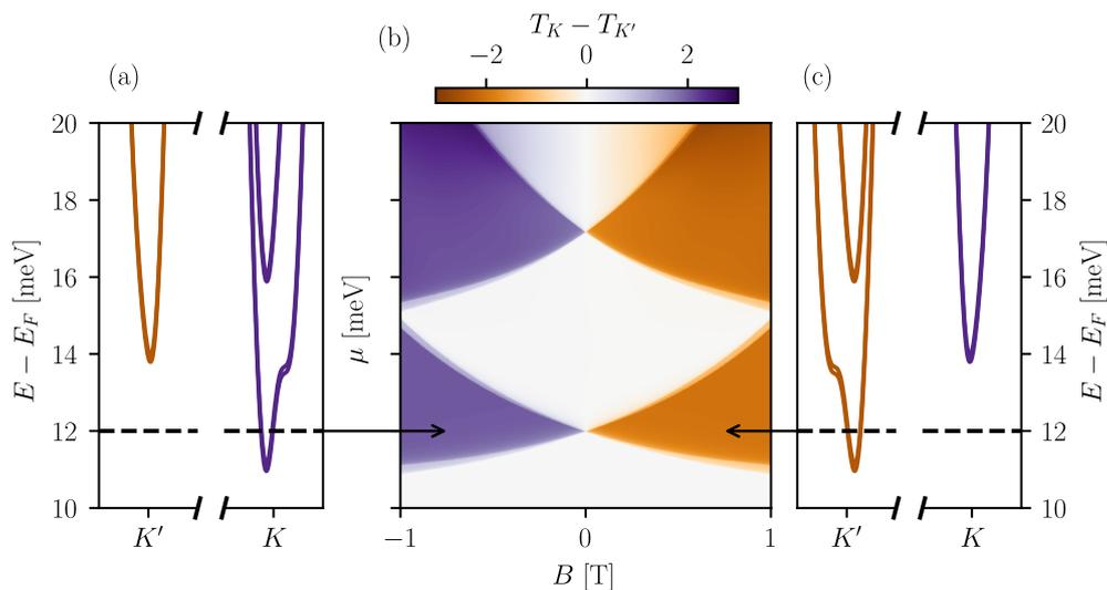
Figure 2: Magnetotransport simulations with a valley splitter. (a, c) Band structure of the injecting arms at finite orbital field  $B$  which lifts the valley degeneracy. As a consequence, the number of propagating modes per valley changes. (b) Transmission difference between the two helical collecting arms. A finite difference indicates the valley polarization of the injected modes. The transmission changes in integer steps, proportionally to the net number of propagating modes per valley.
