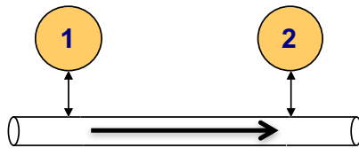
Figure 7: Schematic showing the basic setup of a cascaded quantum system, where two quantum systems interact via a unidirectional (i.e. “chiral”) waveguide. In the Markovian limit, the interactions mediated between the two systems via the waveguide correspond exactly to our effective directional Lindblad master equation.
