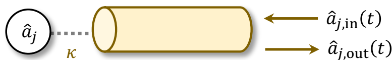
Figure 2: Schematic showing a single cavity (lowering operator \hat{a}_j ) coupled to an input-output waveguide or transmission line. \hat{a}_{j,\text{in}} encodes the amplitude of signals and noise incident on the cavity, whereas \hat{a}_{j,\text{out}} encodes the amplitude of signals and noise leaving the cavity.
