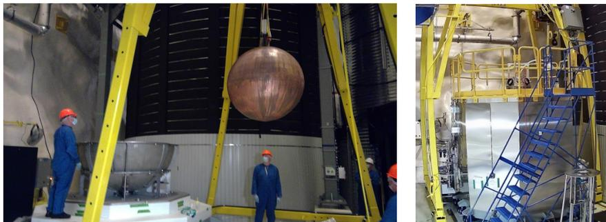
Figure 2: Left: The 140 cm in diameter NEWS-G spherical proportional counter being installed in SNOLAB. Right: The detector's shielding. The shield is comprises 3 cm archeological lead, 22 cm low activity lead, and 40 cm high-density polyethylene, encased in a stainless steel skin.
