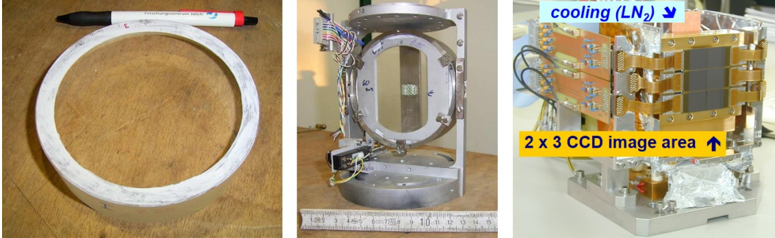
Figure 14.2: Left: quartz disk attached adhesively to a concave glass lens, middle: crystal mounting in an adjustable support frame with an aperture to limit the so-called Johann defocussing, right: focal-plane X-ray detector removed from the cryostat [13].
