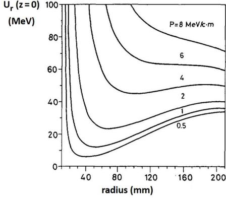
Figure 13.1: Radial distribution of the quasipotential in the median plane for different positive values of the generalized momentum  $P$ .
