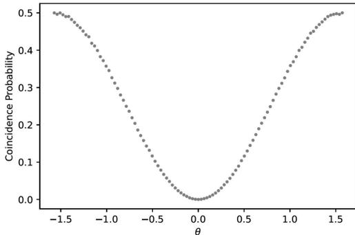
FIG. 7: HOM dip classical simulation graph according to variation of  $\theta$  from  $-\pi$  to  $\pi$ . The interval between angles is  $\pi/100$ . All simulations were performed using Qiskit’s qasm\_simulator.
