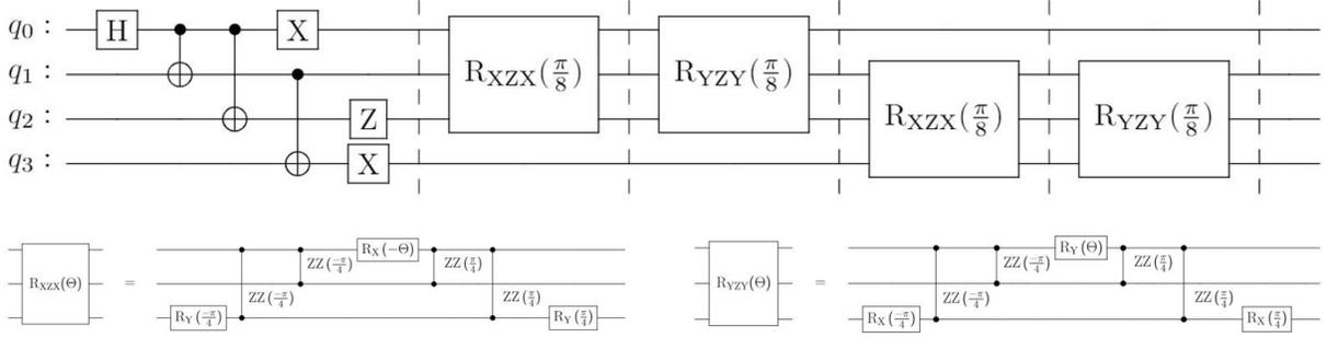
FIG. 4: Full circuit for HOM experiment. As seen in figures in the second line,  $T_H$  given by Eq. (32) is further decomposed into one- or two-qubit gates. We set, for example,  $R_{XZX}(\Theta) = \exp[i\Theta(X \otimes Z \otimes X)]$ , where the index indicates the operator in the exponent.
