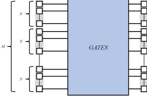
FIG. 3:  $NM$  qubits that can simulate  $N$  bosons in  $M$  modes. Each bundle of  $N$  qubits behaves as a mode that can contain up to  $N$  bosons. Using  $M$  bundles of  $N$  qubits, we can simulate  $N$ -boson scattering process in  $M$  modes.
