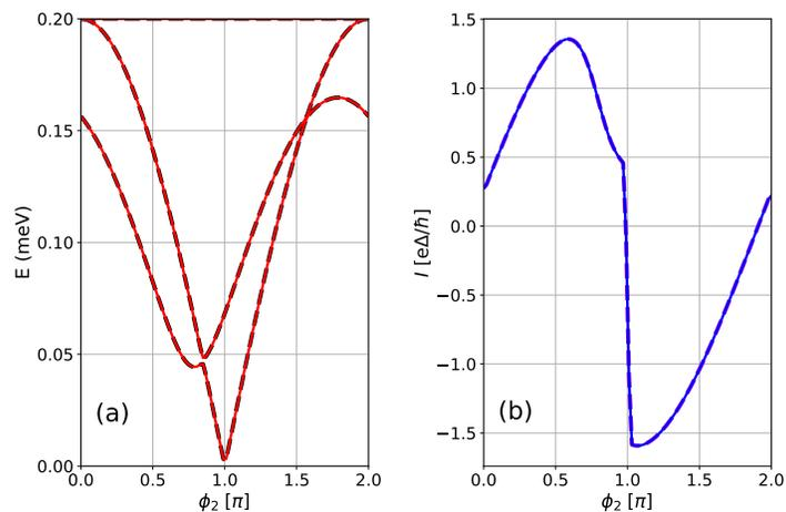
Figure 1: ABS spectra (a) and Supercurrent (b) with the effect of Zeeman interaction included (red and blue solid line respectively). Dashed lines represent the case without Zeeman effect
