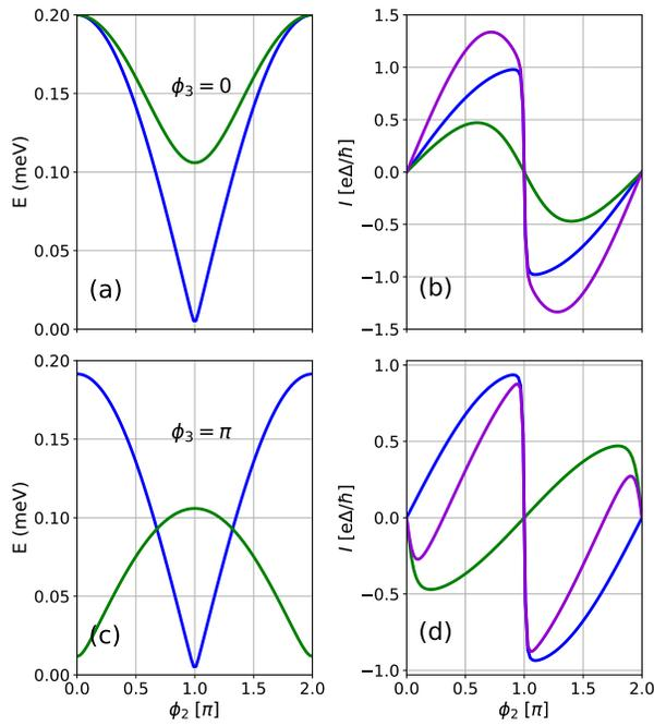
Figure 2: Top panels: energy spectrum (a) and supercurrents (b) in three-terminal Josephson hosting two ABSs for  $\phi_3 = 0$ . Bottom panels: energy spectrum (c) and supercurrents (d) for  $\phi_3 = \pi$ . The other parameters are the same as in Fig. 2 of the manuscript.
