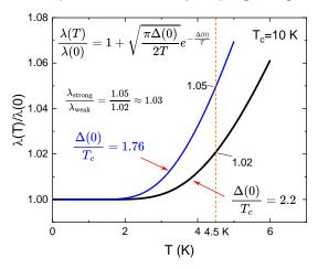
The x-axis is in actual degrees and the y-axis is calculated with the asymptotic formula shown. The blue curve is the weak-coupling limit, and the black curve is calculated for the enhanced gap to Tc ratio. From this, we estimate that at T=4.5 K, the ratio of London penetration depths is 1.03, where the strong coupling value is slightly larger.
