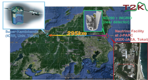
Figure 2: Geographical view of the T2K experiment layout.
