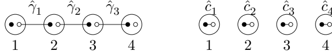
Figure 6: Left: an L = 4 open chain with the off-site Majorana pairing leading to the Bogoliubov vacuum. Right: The on-site Majorana pairing leading to the ordinary vacuum for h_j > 0 .
