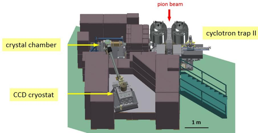
Figure 14.1: Set-up in the  $\pi E5$  area at PSI. The Bragg crystal is mounted inside a vacuum chamber and connected to the cyclotron trap and the CCD X-ray detector by a vacuum system to minimize absorption losses. The roof of the concrete cave is not shown.
