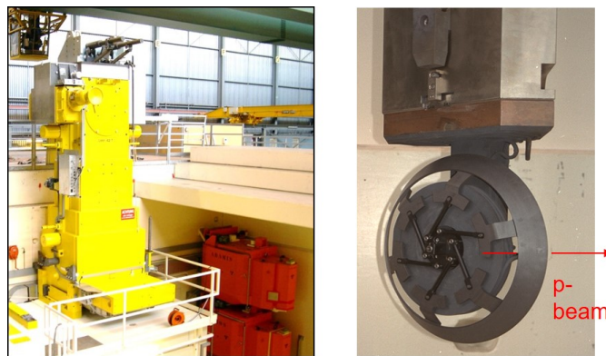
Figure 3.1: Left: Exchange flask (yellow) for the Target E insert. In the background in orange is the exchange flask of Target M. Right: Target E insert with the old graphite wheel design.
