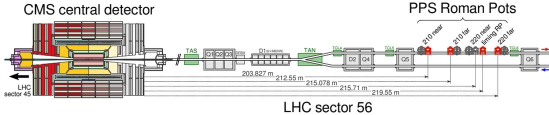
Figure 1: Schematic layout of the beam line between the interaction point and the RP locations in LHC sector 56, corresponding to the negative  $z$  direction in the CMS coordinate system and the outgoing proton in the clockwise beam direction.
