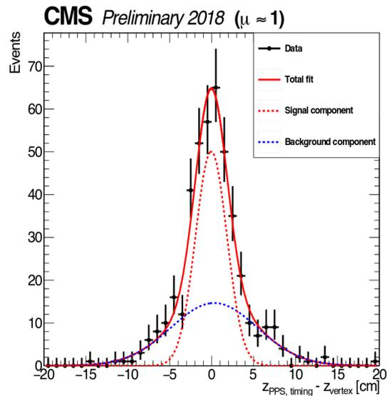
Figure 5: PPS vertex measurement resolution, defined as the difference between vertex position measured by CMS ( $Z_{CMS}$ ) and that calculated from the protons time of arrival in PPS ( $Z_{PPS}$ ). The red curve shows the fit to the signal component, the blue curve that to the background shape [6].
