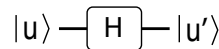
Figure 1: Quantum circuit for a single qubit, where a single Hadamard gate transforms |u\rangle to |u'\rangle = H|u\rangle .
