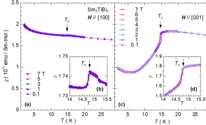
Figure 2: (a) (b) Temperature dependences of magnetic susceptibility of  $\text{Sm}_3\text{TiBi}_5$  below 30 K at applying several magnetic field. (c) (d) Inset shows an enlarged view near  $T_x$ .
