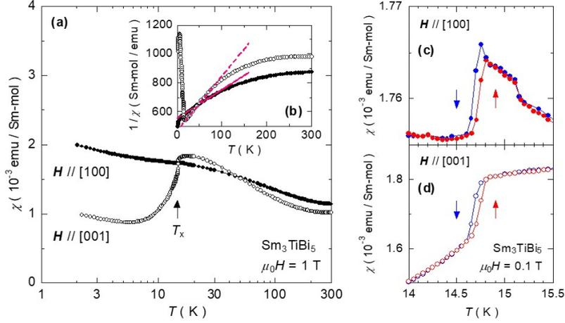
Figure 1: Temperature dependences of (a) magnetic susceptibility and (b) reciprocal susceptibility of  $\text{Sm}_3\text{TiBi}_5$  at  $\mu_0H = 1$  T. The solid and dashed lines indicate Curie-Weiss fitting within  $T = 30$  K to 80 K in Fig. 1(b). Temperature dependences of magnetic susceptibility of  $\text{Sm}_3\text{TiBi}_5$  near  $T_x$  in the magnetic field direction along (c) [100] and (d) [001].
