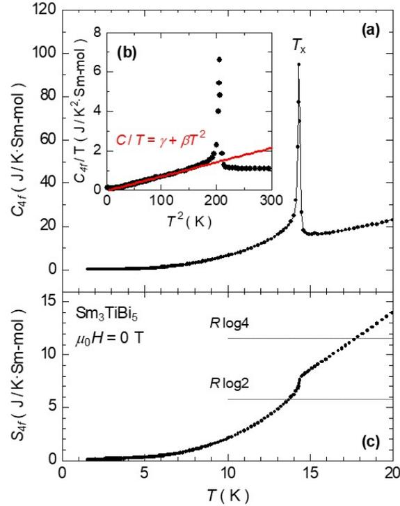
Figure 4: (a) Temperature dependence of specific heat of  $\text{Sm}_3\text{TiBi}_5$  at zero magnetic field. Only the 4f electron contribution component is plotted in this graph. (b)  $C_{4f}/T$  vs  $T^2$  plot of the result of Fig. 4(a). The solid line indicates a  $T^2$  fitting. (c) Temperature dependence of magnetic entropy estimated from the result of Fig. 4(a).
