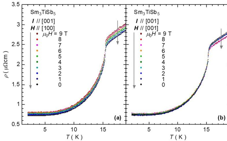
Figure 6: Temperature dependences of electrical resistivity of  $\text{Sm}_3\text{TiSb}_5$  at applying several magnetic field up to 9 T along the direction (a) [100] and (b) [001].
