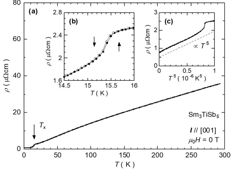
Figure 5: (a) Temperature dependence of electrical resistivity of  $\text{Sm}_3\text{TiSb}_5$  at zero magnetic field. (b) An enlarged view near  $T_x$ . The solid and open circles are corresponding to heating and cooling, respectively. (c)  $\rho$  vs  $T^5$  plots below 16 K.
