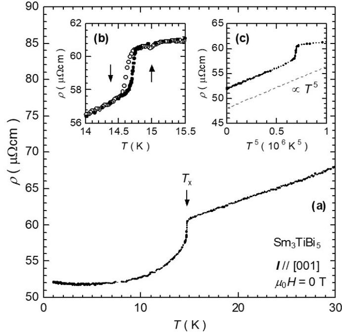
Figure 3: (a) Temperature dependence of electrical resistivity of  $\text{Sm}_3\text{TiBi}_5$  at zero magnetic field. (b) An enlarged view near  $T_x$ . The solid and open circles are corresponding to heating and cooling, respectively. (c)  $\rho$  vs  $T^5$  plots below 16 K.
