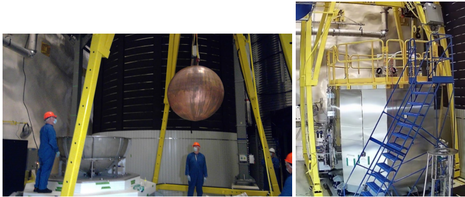
Figure 2: Left: The 140 cm in diameter NEWS-G spherical proportional counter being installed in SNOLAB. Right: The detector’s shielding. The shield is comprises 3 cm archeological lead, 22 cm low activity lead, and 40 cm high-density polyethylene, encased in a stainless steel skin.
