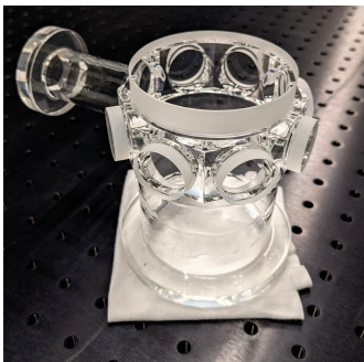
Figure 5: The microscope cell . Manufactured from quartz glass (body) and fused silica (windows). Polished faces on left and bottom tube are for indium sealing. The viewports feature a broadband, broad-angle, gradient-index nanostructure coating on the inside. For scale, the hole distance in the breadboard below is 25 \text{ mm} .
