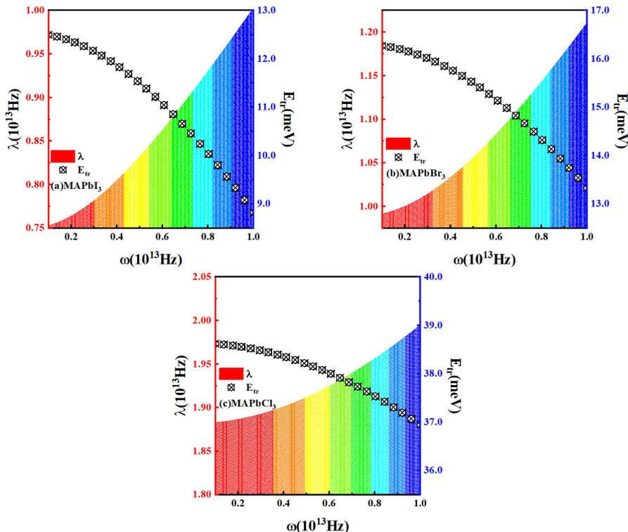
Fig. 2: The vibration frequency and self-trapping energy are linearly correlated with confined strength of parabolic potential. (a)MAPbI<sub>3</sub>. (b)MAPbBr<sub>3</sub>. (c)MAPbCl<sub>3</sub>.
