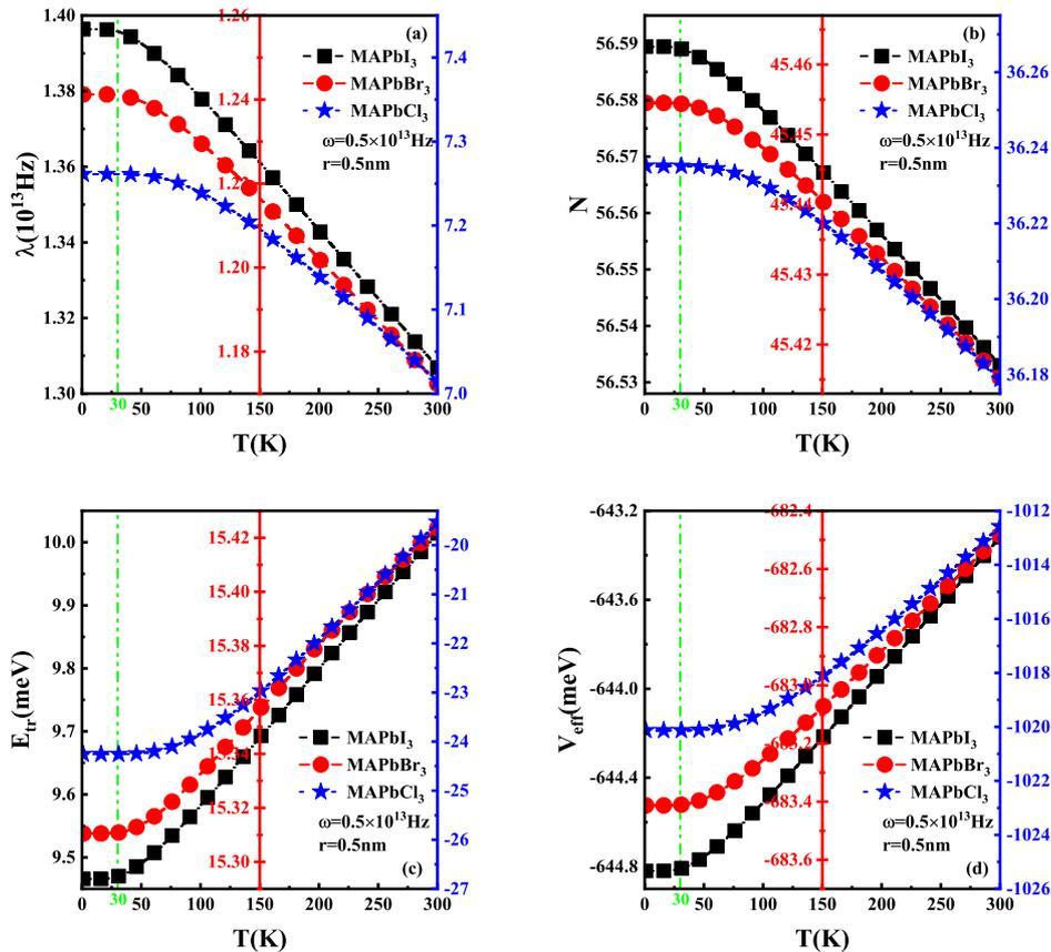
Fig. 4: The (a) vibration frequency, (b) LO-phonon mean number, (c) self-trapping energy, and (d) effective potential energy are linearly correlated with temperature.
