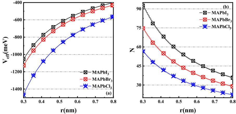
Fig. 3: The (a) effective potential and (b) LO-phonon mean number are linearly correlated with internal relative motion coordinates of bipolaron.
