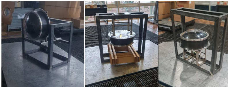
Figure 4: mPMT and support structures vibration test for the top, bottom and barrel positions. Copyright our own.
