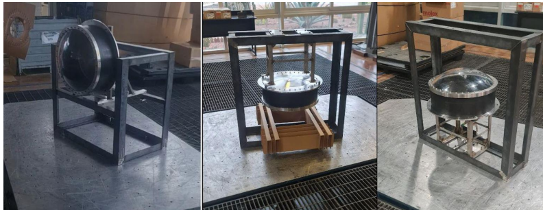
Figure 4: mPMT and support structures vibration test for the top, bottom and barrel positions.
