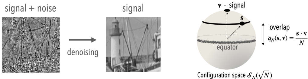
Figure 2: Left. An example of denoising problem: an instance of an image (the signal) corrupted by noise is presented, and the goal is to recover the signal. Figure adapted from [11]. Right. Sketch of the configuration space associated to the denoising problems discussed in these notes, the hypersphere \mathcal{S}_N(\sqrt{N}) embedded in \mathbb{R}^N . The signal is a high-dimensional vector \mathbf{v} ; the portion of configuration space that is orthogonal to the signal is referred to as the equator in these notes.
